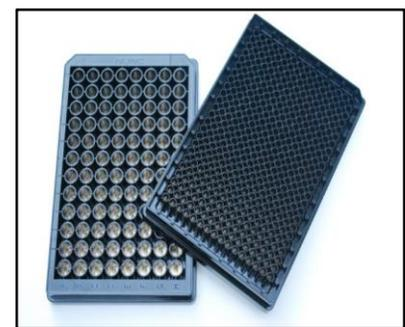
Electrokinetically-enabled microtiter plates ("iPlates") **replace** conventional micro-plates as reaction vessels. Laboratory workflow is unchanged.
